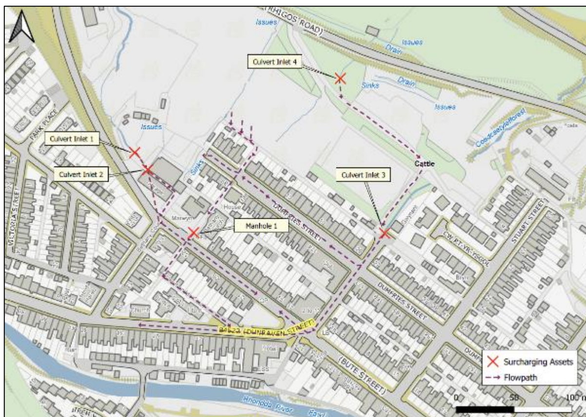
Figure 4: Observed flow paths within 'Treherbert West' sub-catchment during Storm Dennis (16 th February 2020)
